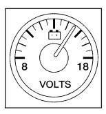
If your vehicle is equipped with the 3800 V6 engine it has a voltmeter gage that indicates battery voltage.
